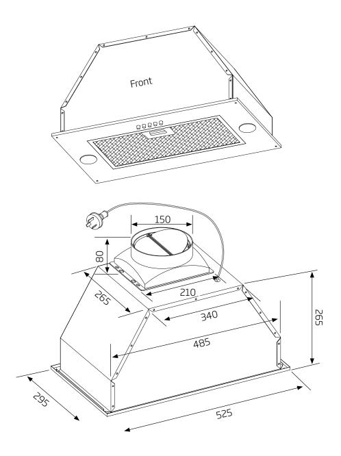
Model: HN-6C, HN-6CB Feeding Voltage: 220-240V 50Hz
