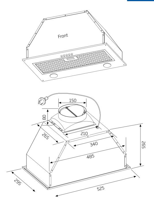
Model: GG-6C, GG-6CB Feeding Voltage: 220-240V 50Hz
