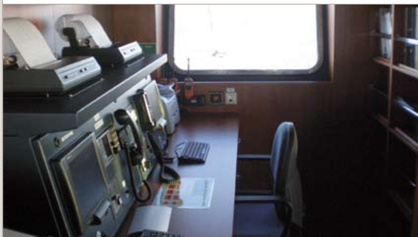
GMDSS Radio Station A3 according to SOLAS/IMO and ITU regulations, ETS and IEC standards
