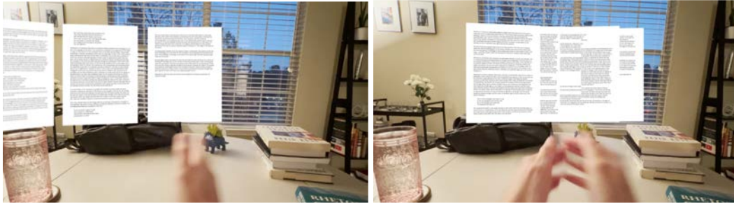
Figure 4.1.2 Full hand swipe from right to left pushes the rightmost papers towards the center of the frame (Left); Both hands brought together merges the paper into a scrollable view (Right).
