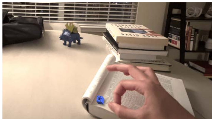
Figure 4.1.14 A 3D QR code with supplementary information is flicked by the user to “send” the digital information to the glasses
