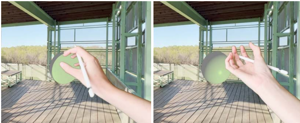
Figure 4.2.7 Cupped hand rotating to create a revolved shape [Note: the gestures have been updated allowing a fist to create a solid revolution and a cupped hand to create a hollow revolution.]
