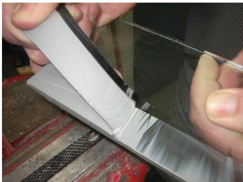
Adhesion to glass or infill panel
