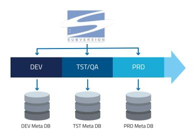
Generally, the above instance propagation strategy is recommended. Depending on the applications in use and the Load, it could be determined to go with a single node deployment or a distributed model deployment. Generally, it is recommended to have a distributed deployment for Production instances. The adapters are forward propagated using the SVN repository.
