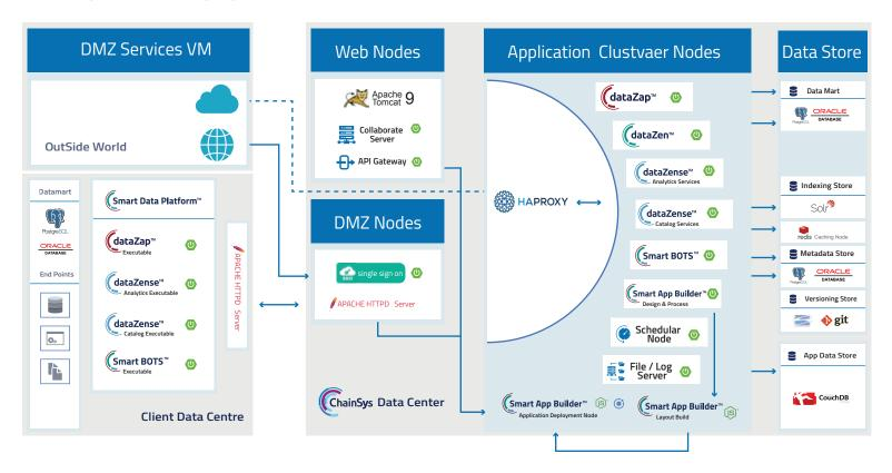
This can be associated along with both the Private or Public cloud. An Agent would be deployed in the client organization's premises or data center to access the endpoints. This would avoid creating the Site to Site tunnel between the Client Data Center and the ChainSys Cloud Data Center.
