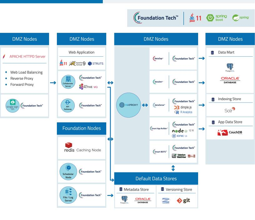
These nodes are generally the only nodes exposed to the external world outside the enterprise network. The two nodes in this layer are the Apache HTTPD server and the "Single Sign O" Node.
