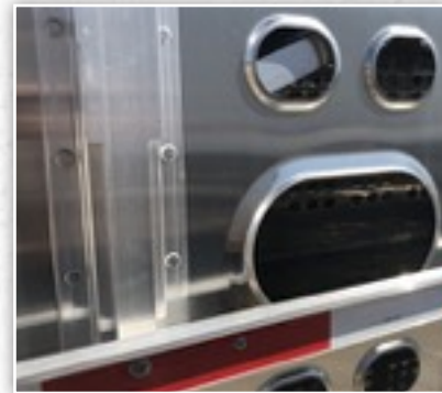
Closure track posts, with tapered notching for easier closure installation
