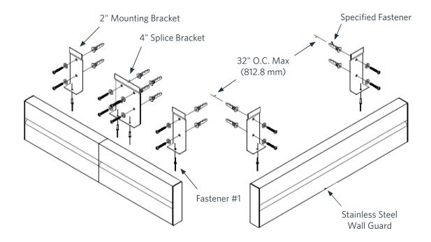
surface for the mounting hardware. See manufacturer's required drill hole sizes as listed on the fasteners (anchors). Note: Observe all safety precautions when drilling to avoid all utilities and re-bar.
