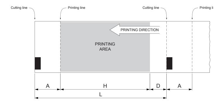
A "Non-printable area" = "Distance between autocutter/printhead"
