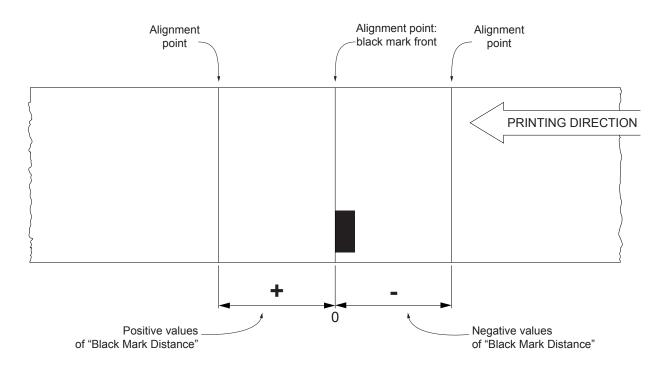
The following figure shows an example of paper with alignment point set by a positive value of "Black Mark Distance" ("Black Mark Distance" = + A):
