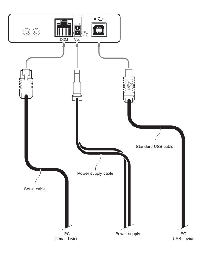
ATTENTION: In some using conditions, we recommend the installation of a ferrite core on the power supply cable.
