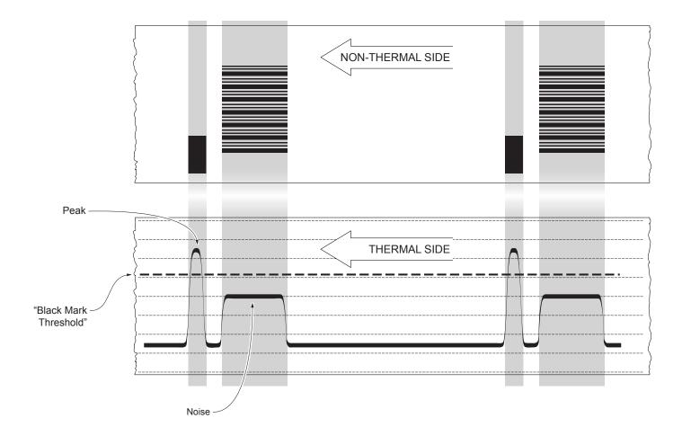
If the maximum value of "noise" read by the sensor is very close to the peak value, it might be difficult to place the value of the "Black Mark Threshold" at an intermediate point. In these cases, it is mandatory that the portion of paper between the point of printing end and the front black mark is completely white (no graphics). In this way, the only next graphic detected by the sensor for alignment after the printing end will be the black mark.
