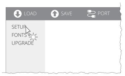
Click on SETUP to access the operating parameteres of the device to be configured.
