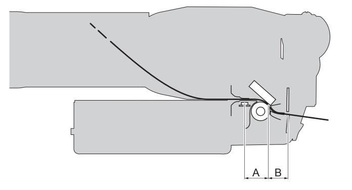
To define the alignment point you need to set the printer parameters that compose the numerical value of the "Black Mark Distance" parameter (see paragraph 6.6).
