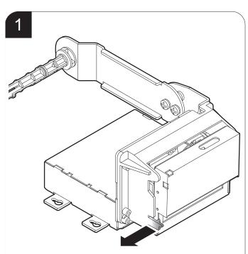
Widen the unlocking hook for the autocutter group.
