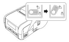
2 While pushing the battery latch, remove the battery.
