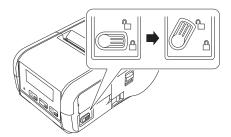
Insert the battery into the battery compartment until the battery latch locks into place. Make sure that the terminal end of the battery is facing inwards and oriented correctly as shown. Do NOT use excessive force to install the battery.
