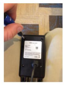
Open the sensor with the T10 screwdriver.
