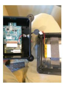
Now that the unit has been completely de-powered, plug it back into the wall and plug in the backup battery. After this is complete, press the black button to put the collector into "pairing mode". This allows it to connect to the sensor and show the RF connection status.
