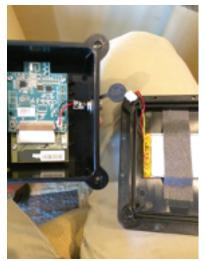
Unplug the backup battery in the collector as well.
