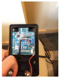
Disconnect the 9v battery from the sensor. Leave the battery unplugged for about 15 seconds. Then plug the battery back in and you should see the lights on the sensor go from Red to Green and then off.
