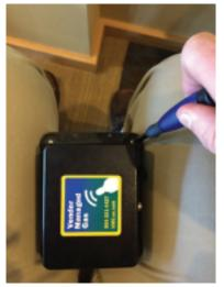
Now, using your T10 bit screwdriver, open the collector.
