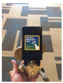
The sensor will be right next to the cylinder(s) in use. It will be on the regulator, C-stic, Cyl-tel box, manifold or inside the Permanent Storage unit.
