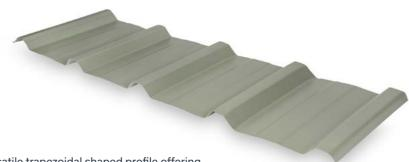
T-Deck is a modern and versatile trapezoidal shaped profile offering excellent strength and spanning capabilities. Manufactured from high-tensile steel, T-Deck is a strong yet lightweight multipurpose profile suitable for commercial, industrial and domestic roofing and walling applications. Available in un-painted zinc/aluminium alloy or a choice of pre-painted colours.
