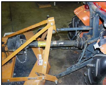
Figure 2. Driveline connected to the tractor
