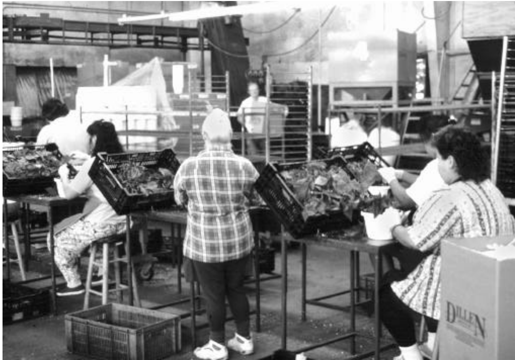
Newly designed stands for potting plants. The stands hold the plant bins at an angle. The slope lets gravity move the plants to the front of the bin so that the plants are always close to the worker and reaching is minimized.
