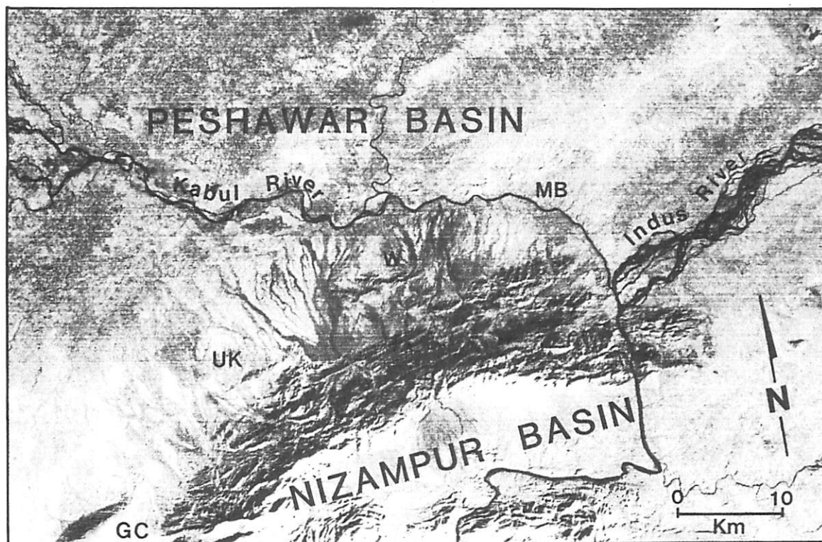
Figure 2. Part of Landsat image 2673-04552-7 of the southern Peshawar basin, acquired 25 November 1976. Note four pressure ridges north of Attock-Cherat Range (GC, UK, W, MB; see Fig. 1), linear fault pattern within the Attock-Cherat Range parallel to faults in these ridges, and absence of linear pattern in Quaternary sediments east of MB.
