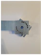
3. Then put the encoder into the slot and then add the wingnut and tighten
