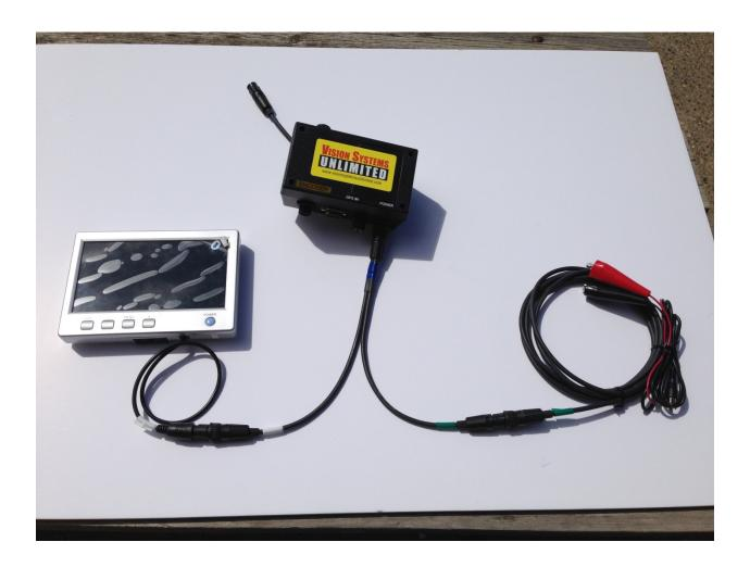
You can control the intensity of the LED lights with the rheostat that is on the top of the control box.
