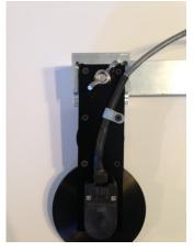
This then clamps onto the Well Casing to hold the pulley over the well.
