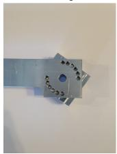
3. Then put the encoder into the slot and then add the wingnut and tighten
