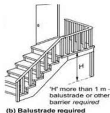
For floors more than 4 m above the surface beneath, any horizontal elements within the balustrade or other barrier between 150 mm and 760 mm above the floor must not facilitate climbing.
