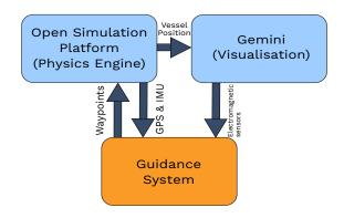
This year's challenge is limited to the guidance system block in the figure above. This module may include systems for sensor processing, state estimation, situational awareness, guidance algorithms and collision avoidance. Teams are not expected to implement control algorithms, as these are outside of the scope of the challenge, and already installed in the simulation platform. Further details of this implementation will be made available when the platform is released.
