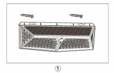
it is recommended to install vertically against the wall 2-3m high above the ground as picture ①shown
