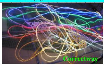
Please note that it can not test the LED strip in roll, otherwise, the inside LED strip will be very hot and will cause the below problem if light up in long time.
