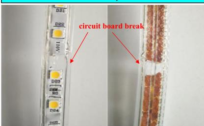
The PVC is stretchable but the Circuit board not.
