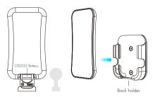
Note: Before the first use, please remove the protective film on the battery.
