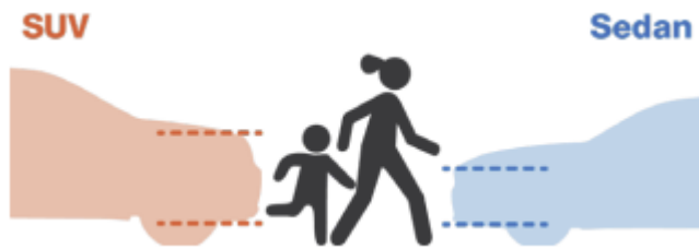
Figure 5: Comparison of vehicle bumper height to pedestrian height
