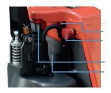
Battery plug--For charging and change battery Emergency button-located where you can easily reach and control, assuring safety for people and truck.
