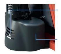
190mm drive wheel make the truck more stable when loading & moving, 48/850W DC Brushless motor is more powerful, maintenance free, big tranmission ratio gearbok, high gradebility, low energy consumption.
