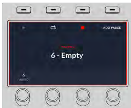
While recording, a red border will appear around the LCD
