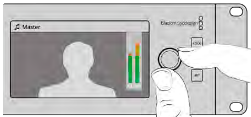
Use the knob to adjust the master audio level and you can see the effect on the main audio meters in the LCD
