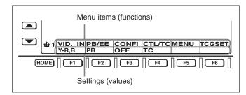
In the figure above, Y-R,B (analog component signals) is selected as the setting for VID.IN, the menu item for button F1. This manual refers to this as "F1 (VID.IN) in function menu HOME page is set to Y-R,B."
