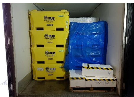
Figure 4. Different packaging used for transporting fresh rainbow trout from Iceland to Poland. The yellow tubs to the left are the 460-L tubs (only the top one with lid), the 250 L tubs are covered with a single, blue plastic cover (pallet cover) and the white EPS boxes at the bottom right.
