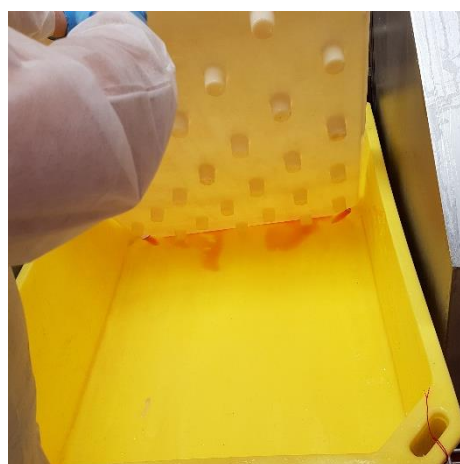
Figure 6. Almost no blood was found on top of or below the drain grid after 8-day storage in the 460 L tub containing 299 kg of fish. Around 10-20 kg of fish could have been packed into the container.
