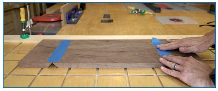
Align the X-PADs' Edge Positioning Guide with the outermost corner of the joints with the Screw Center Guide off the edge of the material, tighten clamps.
