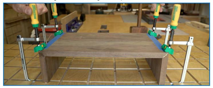
Use a machinisht square to ensure that the sides are 90-degrees with the top. If necessary, lightly tap the sides with a non-marring mallet to square them up with the top.
