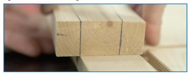
Once your workpiece is aligned, place the slotted stops up against two sides of the workpiece and lock them in place with **MATCH**FIT Dovetail Hardware. Make sure that every piece is contacting the stops to ensure uniformity. Clamp workpiece in place with **MATCH**FIT Dovetail Clamps and advance sled along the fence through the cut.
