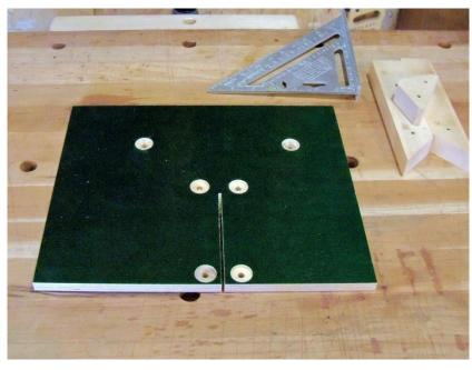
A square is used to align the cleats so that they form a perfect 90 degree angle. Loosen the rear bolts and the oversized holes in the cleats will allow for adjustment. Set the screws tight when you have them aligned. You want the 90 degree cleats to be as close to 45 degrees to the kerf as possible, but the 90 degree angle is the most critical.
