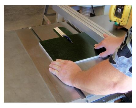
before we can proceed. Set the rip fence to hold the sled evenly spaced over the miter slots and cut a kerf about 1/3 of the way into the base plate.
