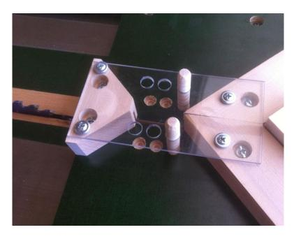
The block behind the cleats will keep the blade covered if the sled is pushed further than needed, but to keep from accidentally over cutting, I prefer to set up the Zero Play Stops that come with the Zero Play Bars.
