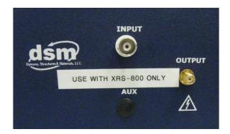
Input and Output Connections on Front Panel of VF-500-XRS with Waveform Generator calibrated for an XRS-800 stage
