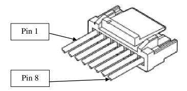
On the GHR-08V-S connector, the pins are numbered such that with the disconnect tab facing UP, pin number 1 is on the far LEFT of the connector.
