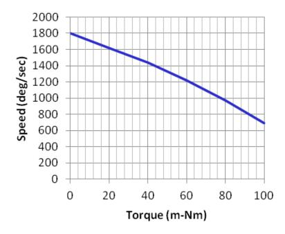
External torque loads above 100 mNm should not be applied to the system, as this may cause backdriving. Backdriving the motor may reduce the overall life of the motor. A backdriving load is distinguished from a frictional load in that a backdriving load attempts to <u>cause</u> motion on the motor output shaft, whereas a frictional load simply <u>resists</u> motion on the motor output shaft.
