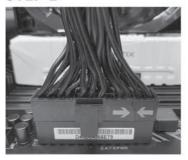
Plug the 24-pin connector onto the motherboard.
