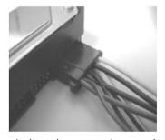
4-pin molex connectors used for hard drive, CD-ROM and cooling fans.
