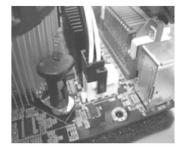
4-pin or 8-pin (4+4pin) + 12V connector used for CPU only.
