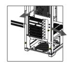
Remove the thumb screw to move the PCI-E slide cover.
