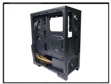
1.4 Make sure that the power supply is correctly installed, and that screw mount points are aligned (as seen in step 1.5).
