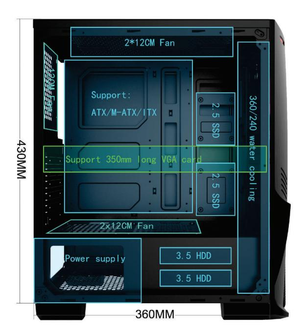
8.1 There is room for up to three 120mm fans or a 360/240mm water cooling setup in the front. There is also room for two 120mm fans in the top, one 120mm fan in the rear, and two 120mm fans in the bottom. You can install up to two 3.5" hard drives and three 2.5" hard drives in the case as well. Supports video cards up to 350mm long. Supports ATX, Micro-ATX, and ITX motherboards.
