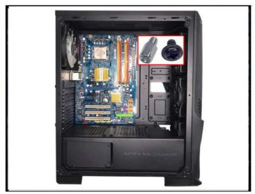
2.3 Align motherboard with standoffs and mount to case. Use the round screws found in the screw bag to secure the motherboard in place.
