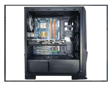
3.2 Read your PCI expansion card's documentation. Install PCI card into correct slot for your card type (x1, x16, etc.). Once the card is seated firmly, secure it with a screw in the appropriate hole. Lower the tab and secure it in place with the screw.
