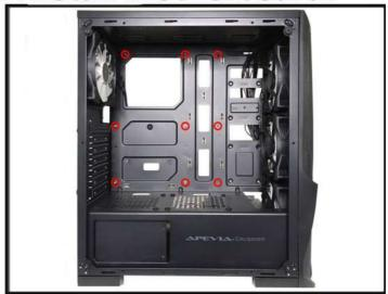
2.1 Most of the mounting holes for the motherboard are already pre-installed, but there are extras just in case they are needed.
