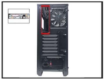
2.2 If your motherboard included an I/O shield, fit the shield in the provided hole on the back of the case until it clicks into place. Make sure that the holes on the shield match up with the I/O connectors on the motherboard.
