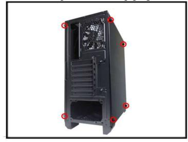
1.1 Remove thumbscrews from both sides of the Crusader case. There are two on the right side (non-window) and four on the right side (window). In order to install all devices, you will have to have access to the entire inside of the case.
