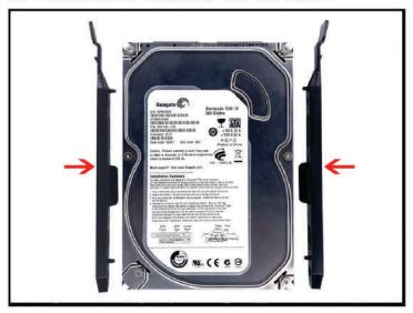
4.1 For 3.5" hard-disk drives, find the mounting rails as shown. Make sure the holes line up and attach them to the drive. Slide them into the drive bay as shown in step 4.3. There is room for up to two 3.5" hard drives.
