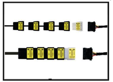
5.1 Four fans are already pre-installed in the case. However, should you need to reconnect them, you need to make sure each of the 4-pin Molex connectors are daisy-chained together as shown above. The one labeled "Isolated Interface" controls the LED pattern/color and needs to plug in directly to the power supply.
