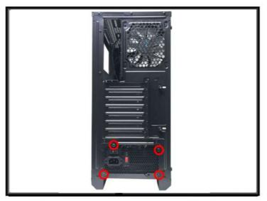
1.5 Fasten screws to the back of the case. Keep a hand on the power supply to keep the holes aligned. It is recommended to install the power supply "upsidedown" (fan pointing towards bottom of case) for better airflow.
