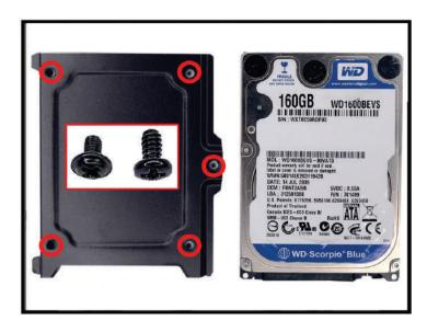
4.2 For 2.5" hard-disk drives, find the mounting bracket as shown on above. Remove the screw and slide the bracket off. Then secure the drive with screws. There is room for up to three 2.5" hard drives.
