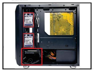
4.3 Original placement of both 3.5" and 2.5" drive mounts are located in the above marked rectangles.
