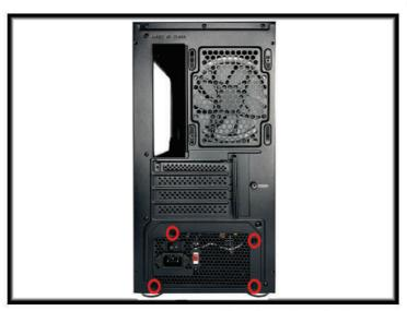
1.5 Fasten screws to the back of the case. Keep a hand on the power supply to keep the holes aligned. It is recommended to install the power supply "upside-down" (fan pointing towards bottom of case) for better airflow.
