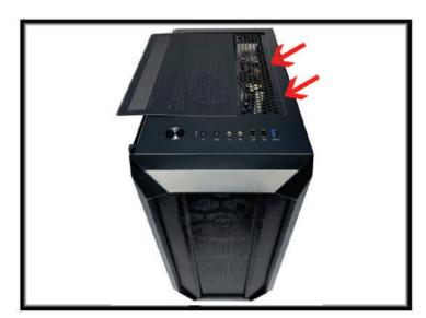
5.3 There is a magnetic filter that sits on the top that allows for easy cleaning. You can remove it by lifting it off and replacing it when it's done. Can be water washed if desired. The switch labeled "RGB" on the top can be pressed to change fan colors or turn them off.
