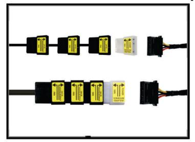
5.1 Three fans are already pre-installed in the case. However, should you need to reconnect them, you need to make sure each of the 4-pin Molex connectors are daisy-chained together as shown above. The one labeled "Isolated Interface" controls the LED pattern/color and needs to plug in directly to the power supply.
