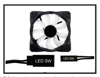
5.2 In order to properly use the colorchanging LEDs on the fans, make sure that one of the male LEDSW connectors from the fans are plugged into the female LEDSW connector coming from the front panel as shown. Hold the RGB button for 3 seconds to reset the pattern.
