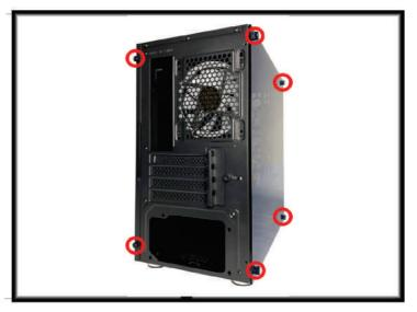
1.2 Grab the notch on the edge of the non-window panel. Pull towards the back to release. Gently remove the glass window by lifting it up. Place both panels to the side until done with the installation process.
