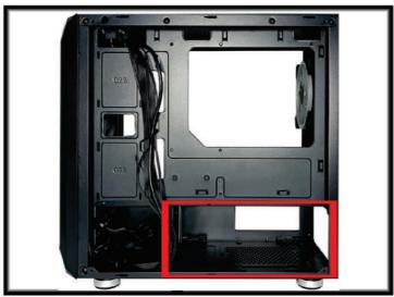
1.3 Install power supply in the spot indicated in the picture. Slide it in until the holes line up in the back.
