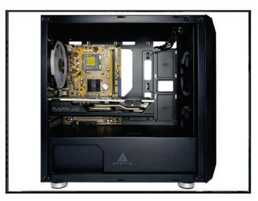
3.2 Read your PCI expansion card's documentation. Install PCI card into correct slot for your card type (x1, x16, etc.). Once the card is seated firmly, secure it with a screw in the appropriate hole. Put the tab back and secure it in place with the screw.
