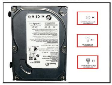
4.1 For 3.5" hard-disk drives, find the two types of screw and the rubber washer as shown above and place the washer to the left side hole. Secure with the nonthumb screw. Slide the drive into the drive bay as shown in step 4.3 then secure with the thumb screw.
