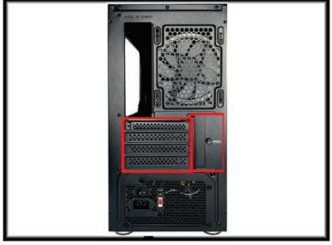
3.1 First, remove the PCI slot covers. Push on the cover at a diagonal angle. Wiggle the cover until it comes loose. Make sure that you remove the correct slot covers as once they are removed you cannot replace them. Make sure you unscrew and remove the tab so you can secure the cards.
