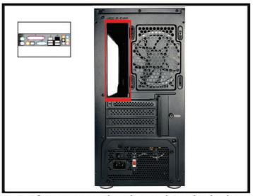
2.2 If your motherboard included an I/O shield, fit the shield in the provided hole on the back of the case until it clicks into place. Make sure that the holes on the shield match up with the I/O connectors on the motherboard.
