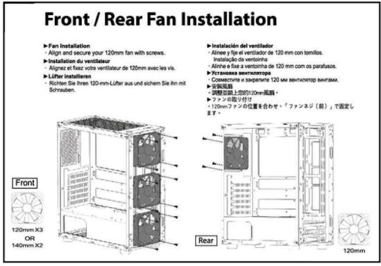
8.1 There is room for up to three 120mm fans or a 360/240mm water cooling setup in the front. There is also room for two 120mm fans in the top, one 120mm fan in the rear, and two 120mm fans in the bottom (bottom fans installed using the long 1 1/4" screws that come in the bag). You can install up to two 3.5" hard drives and two 2.5" hard drives in the case as well. Supports video cards up to 350mm long. Micro-ATX, and ITX motherboards.
