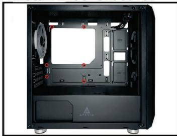
2.1 Most of the mounting holes for the motherboard are already pre-installed, but there are extras just in case they are needed.
