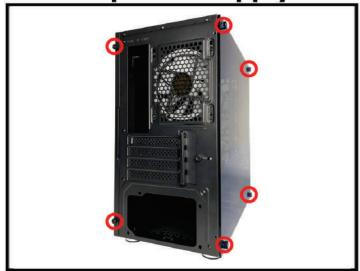
1.1 Remove thumbscrews from both sides of the Prodigy case. There are four on the window and two on the solid side panel. In order to install all devices, you will have to have access to the entire inside of the case.
