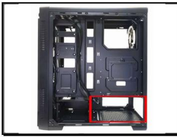
1.3 Install power supply in the spot indicated in the picture. Slide it in until the holes line up in the back.
