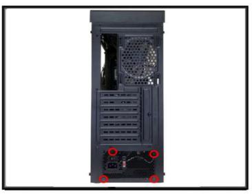
1.5 Fasten screws to the back of the case.
