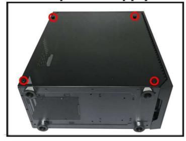
1.1 Remove thumbscrews from both sides of the Trinity case. There are four on each window sides. In order to install all devices, you will have to have access to the entire inside of the case.
