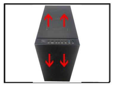
5.3 In order to replace the fans in the top, you need to remove the front panel first by pulling it off, then the top by pulling it up. The fans themselves are secured on the under side of the case frame. The button on the top labeled "LED" can be pressed to change fan colors or turn them off.
