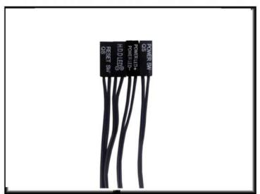
6.1 Locate the above front panel leads. Refer to your motherboard user's manual for placement schematics.
