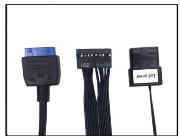
6.2 Locate the above front panel leads. Your motherboard user's manual will provide schematics. The triangular markings ▲ on the leads indicate positive wires. The 4-pin Molex connector for the front panel logo LED goes to the power supply.
