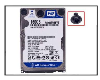
4.2 For 2.5" hard-disk drives, find the mounting screws as shown above. Secure the drive with these screws to the bays as seen in Step 4.3. There is room for up to two 2.5" hard drives.
