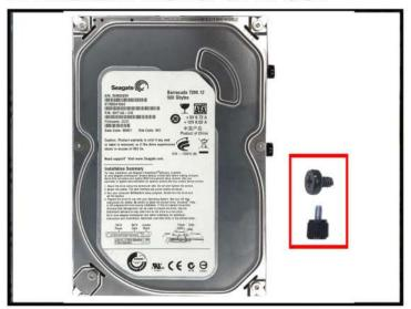
4.1 For 3.5" hard-disk drives, find the smaller thumb screws (above top) and secure them to the two top holes of the drive. Slide the drive into the drive bay as shown in step 4.3 then secure with the bigger thumb screw (above bottom). There is room for up to two 3.5" hard drives.
