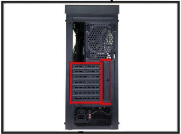
3.1 First, remove the PCI slot covers. Push on the cover at a diagonal angle.
