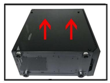
1.2 Gently remove each glass window by lifting it up. Place both panels to the side until done with the installation process.
