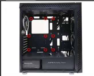
2.1 Most of the mounting holes for the motherboard are already pre-installed, but there are extras just in case they are needed.
