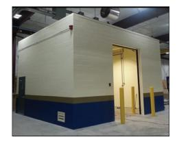
The overall footprint is 87" wide x 54" deep x 96" high. It contains the test stand, which is 48" wide x 48" deep x 96" high; the test chamber itself where the actual testing is done is 40" x 40" x 40". Front and top doors are manually opened for the installation and removal of the swivel assemblies. The test chamber is enclosed using polycarbonate sheet and expanded flattened sheet metal on all sides. There's also three electric motor hydraulic pump units.
