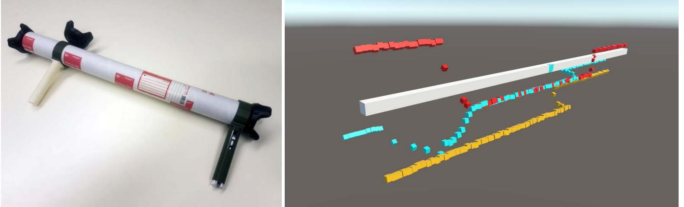
Fig. 1 The tangible pipe input device showing two handles with button input, and the matching VR view of the data along the pipe's axis (shown in white).
