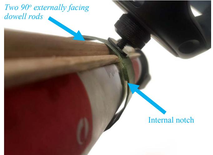
Fig. 6 The physical locking mechanism on the pipe consisting of two 90° sections of dowel, and notch on the inside of the ring.
