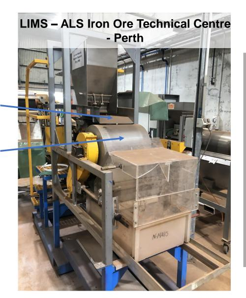
Low Intensity Magnetic Separation (LIMS) processing trials were performed to give a first pass indication of upgradability of crushed drill core samples.
