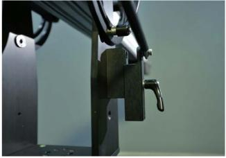
Mount parallelogram rod conclusive if camera Mount parallelogram rod not conclusive, if should be horizontal while tilting Mutiglider. camera should tilt while tilting Multiglider.
