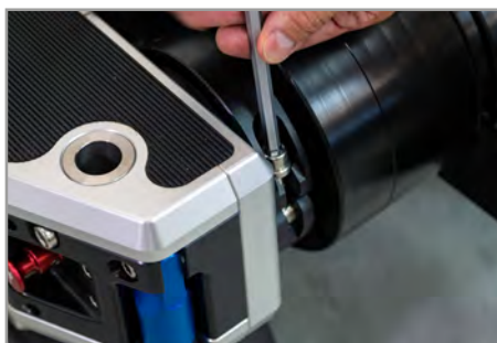
Open the two screws on the left and right side of the scissors-arm (front side of the dolly) with the integrated Allen Key.
