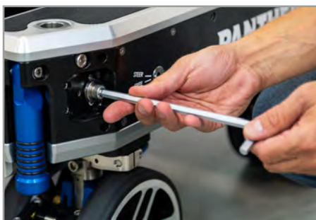
Open the mechanical connection screw on the side of the dolly with the integrated Allen Key.
