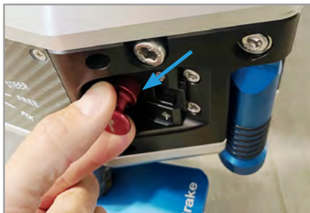
Disconnect the red electricity knob by pulling it out.
