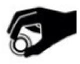
The emergency push button (Ref.37) must be used ONLY in case of emergency. If activated, it must be unblocked turning it clockwise.
