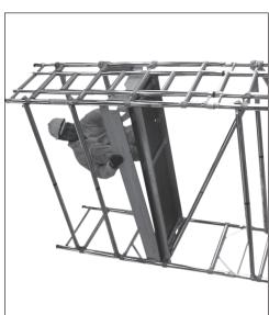
platforms, handrails, mid rails and toeboards must be fitted.
