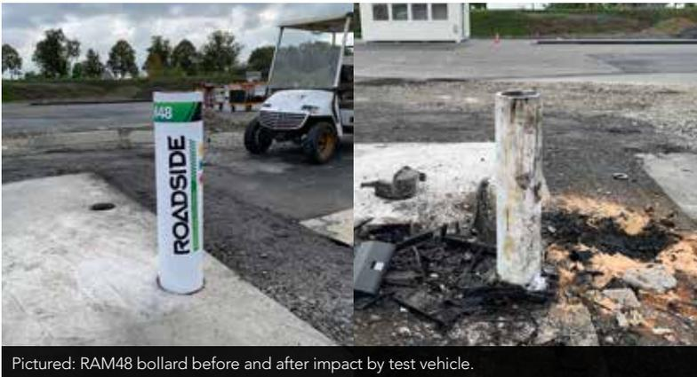
Pictured: RAM48 bollard before and after impact by test vehicle.
