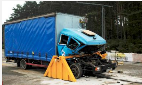
VSB Gate: Narrow impact point will focus energy into the occupant compartment causing undue risk to errant vehicles. This device should be located such that it cannot be impacted by errant vehicles.
