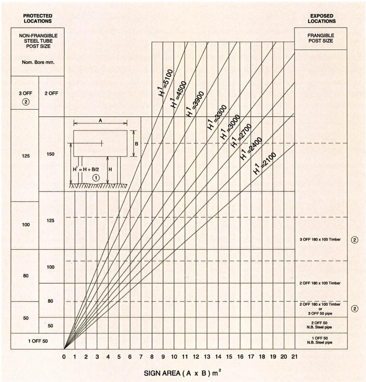
Figure 6.1: Sign Post Selection Guide (All dimensions in millimetres otherwise shown)
