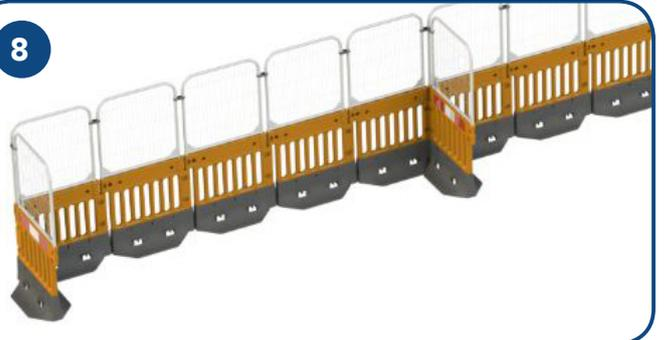
For wind speeds over 40mph brace the barrier configuration with 1 StrongFence for every 5, connected via a fence clamp.
