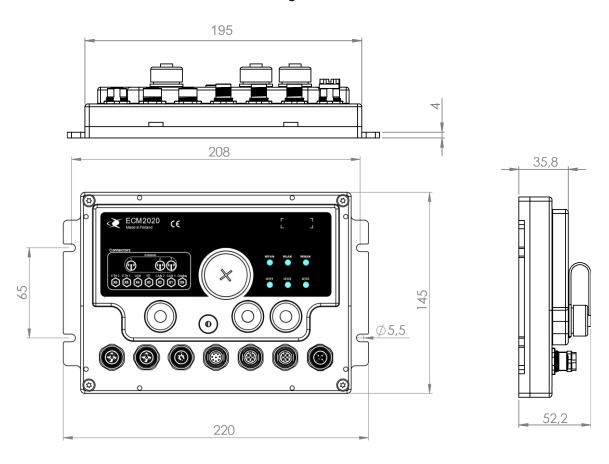
The preferred mounting position is connectors pointing downwards. If the unit is mounted connectors pointing to the side, then it is vital to leave some loose cable with a downward cue to prevent the ingress of moisture through connector.
